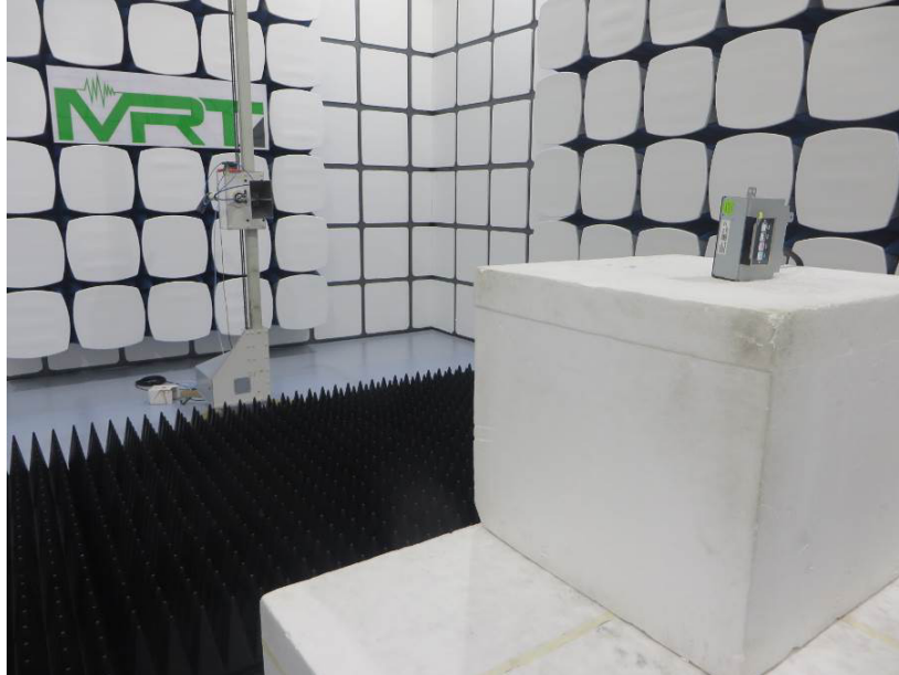
Photograph 3: Set-up for Radiated Test above 1GHz
