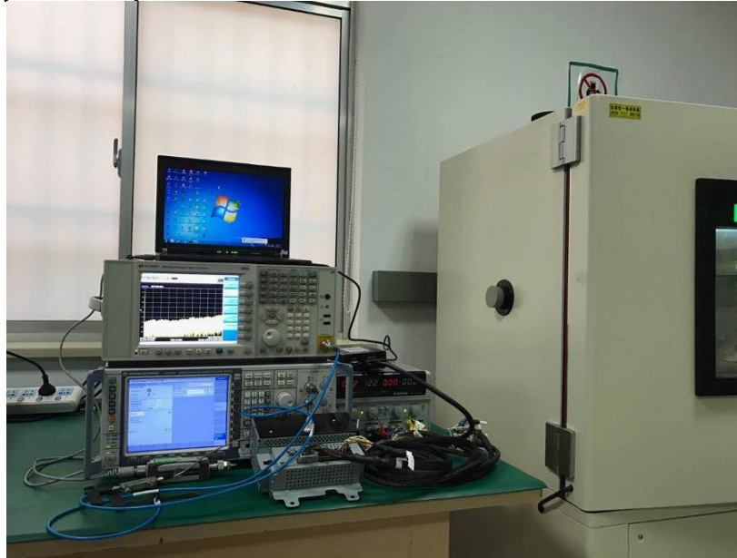
Photograph 1: Set-up for Conducted Test
