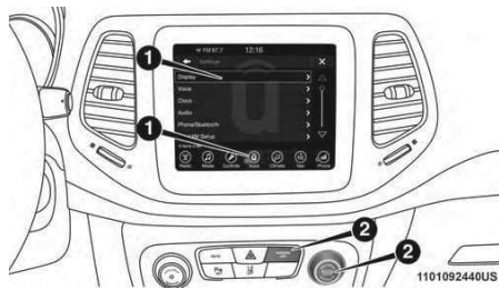
1 — Uconnect Buttons On The Touchscreen 2 — Uconnect Buttons On The Faceplate
