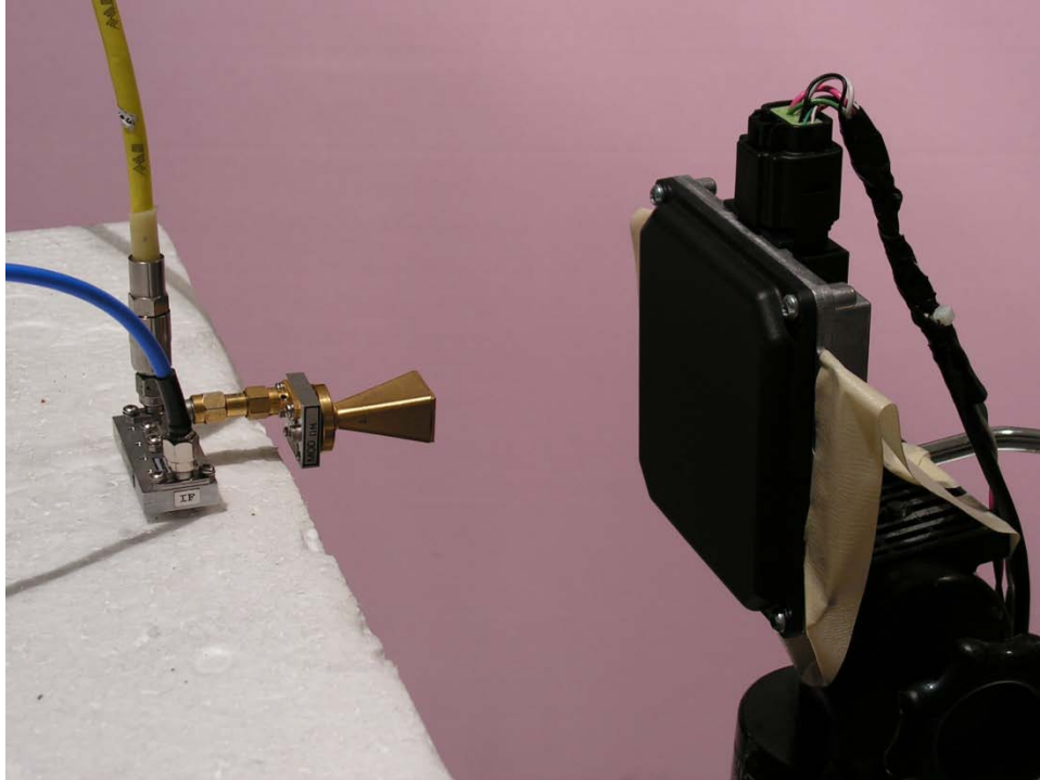
High Frequency DUT test setup (one of three axes tested)
