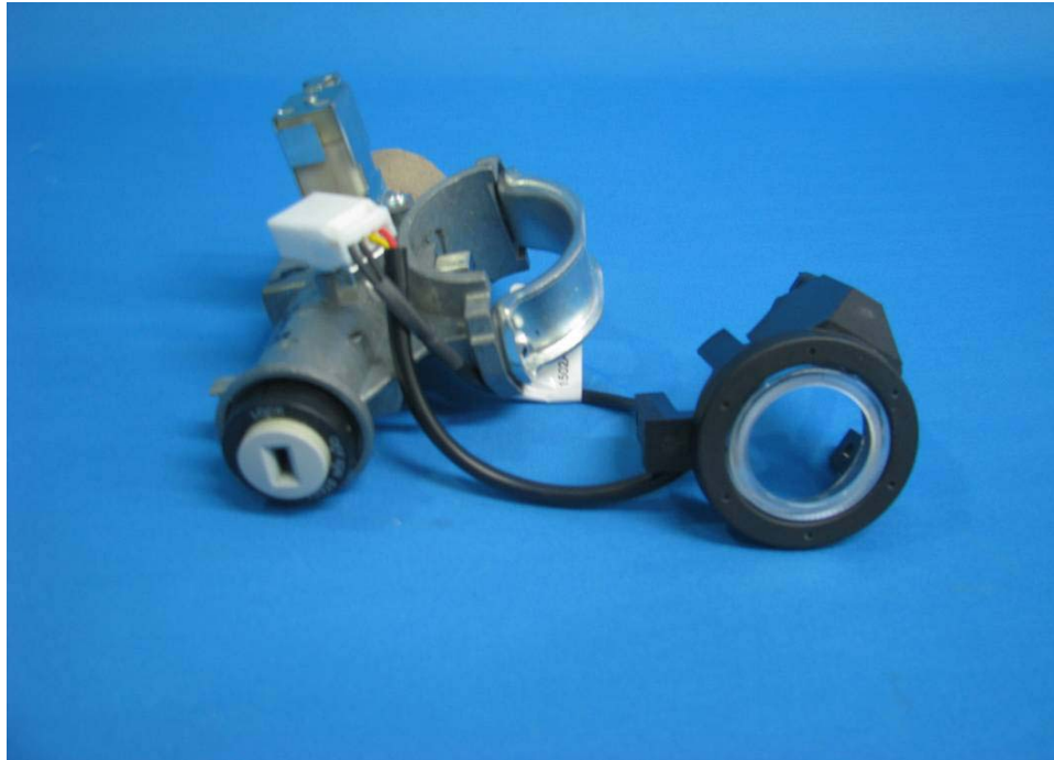
EUT Overall View with RFID Coil removed
