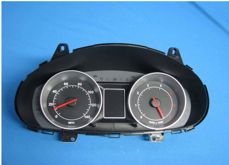
Cluster – Top Cover removed
