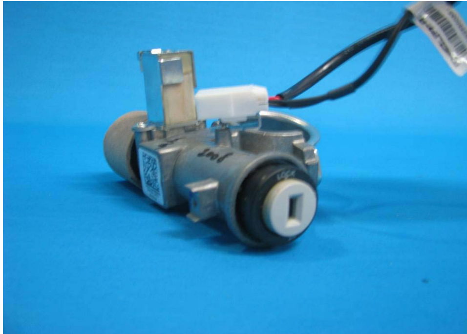
EUT Lock – With RFID Coil removed
