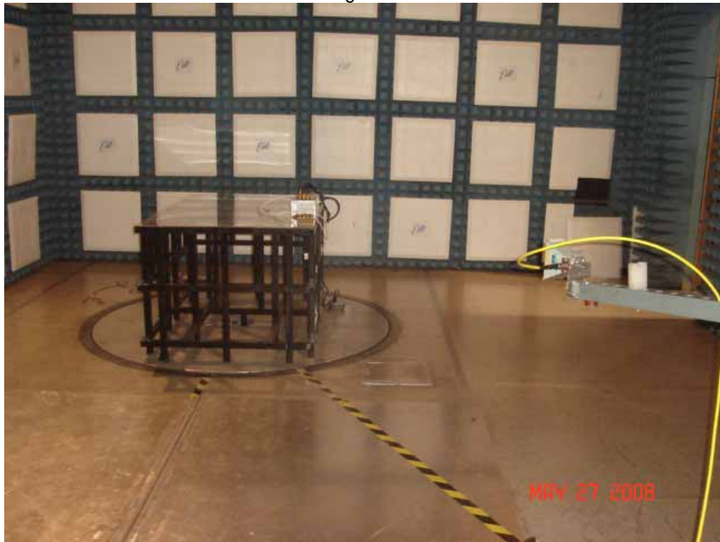
Test Set-up for Radiated Emissions – Horizontal Polarization
