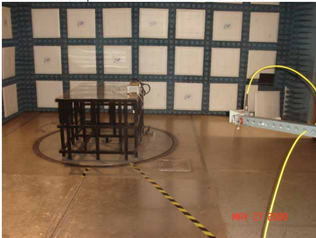
Test Set-up for Radiated Emissions – Vertical Polarization
