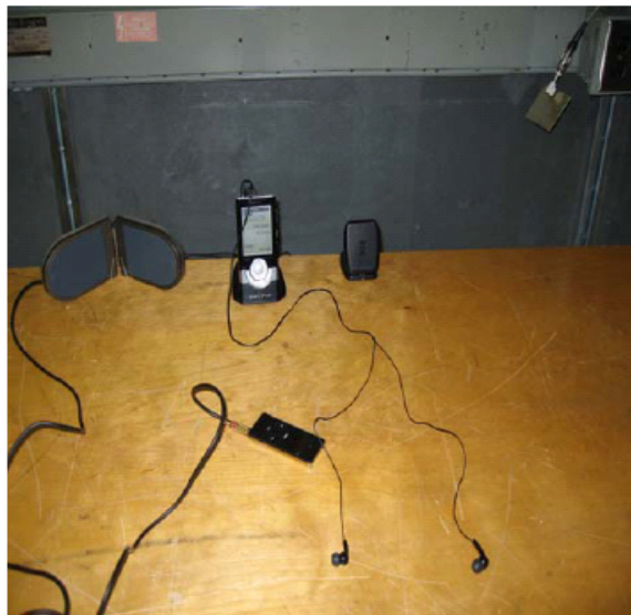
Photograph 2 : Test Setup for Conducted Emissions
