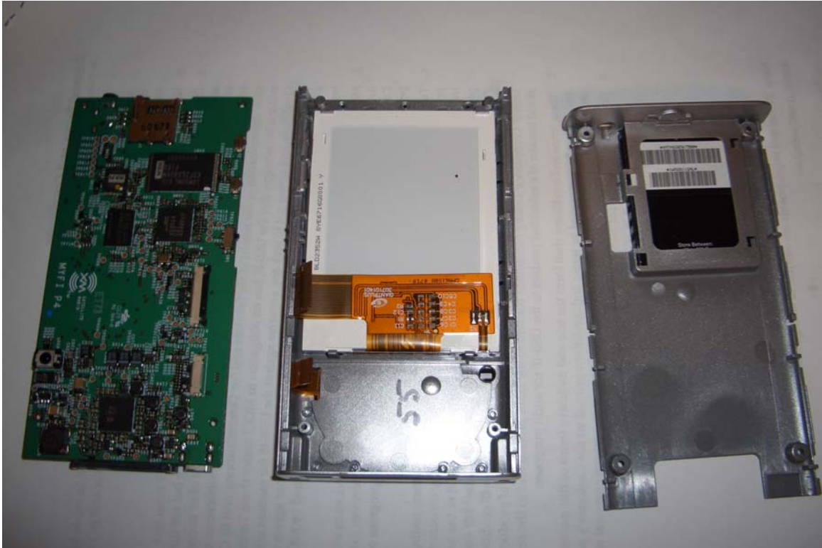
Figure 3: Battery frame, display section and digital side of board
