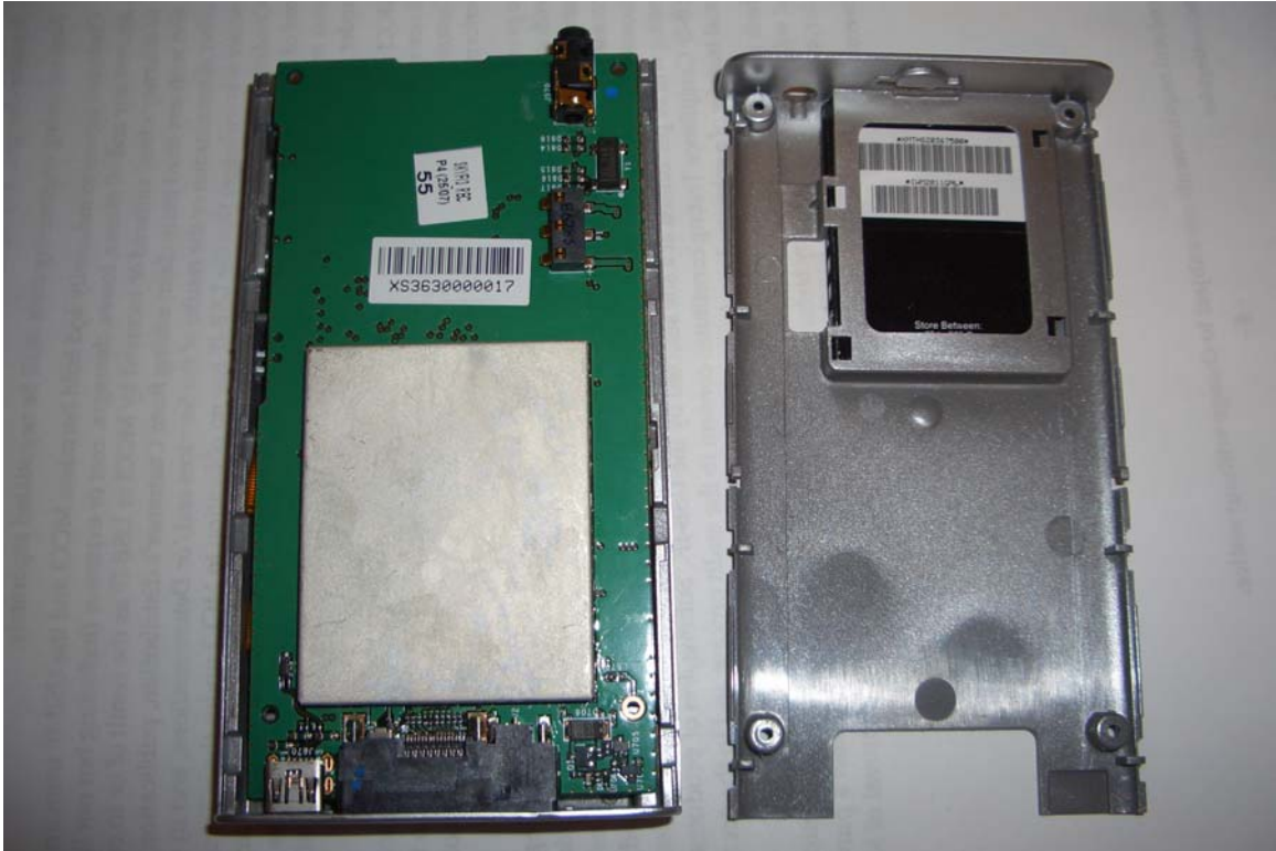
Figure 1: Battery Frame on right, Circuit board showing RF section
