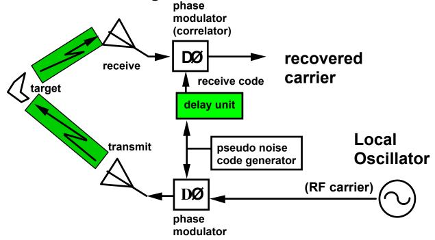
When the internal delay of the receive code matches the time of flight to target and back, receiver output is at a maximum as governed by return target signal power
