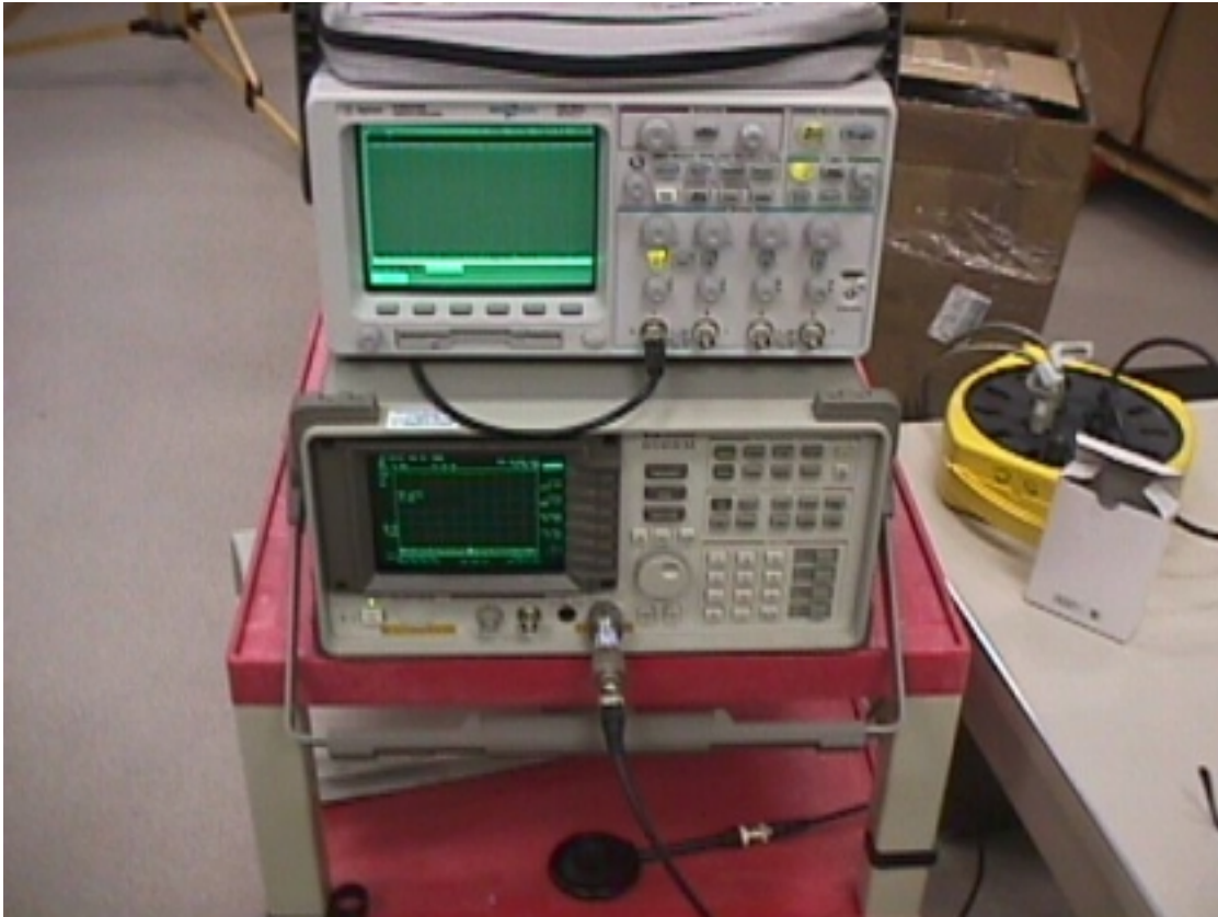
View of the Agilent (HP) model 54624A 100 MHz digital oscilloscope; HP 8591EM spectrum analyzer; and EMCO 7405-901 6 centimeter H field probe, used to create the data packet detail plots.
