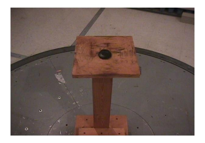
View of the Delphi HDNA transmiter during the Radiated Emissions tests. This view shows the orientation of the product where the maximum signal levels were present (horizontal polarity).
