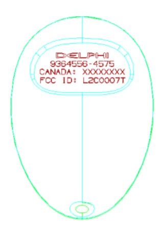
RFA-X FOB Back Cover Label Detail (molded into back cover)
