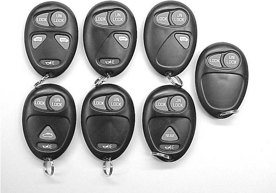
RFA-X FOB Group of Seven Different Production FOBS (Circuit boards are identical for all versions)
