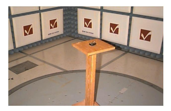
View of the Delco J/Z transmiter during the Radiated Emissions tests. This view shows the orientation of the product where the maximum signal levels were present (horizontal polarity).
