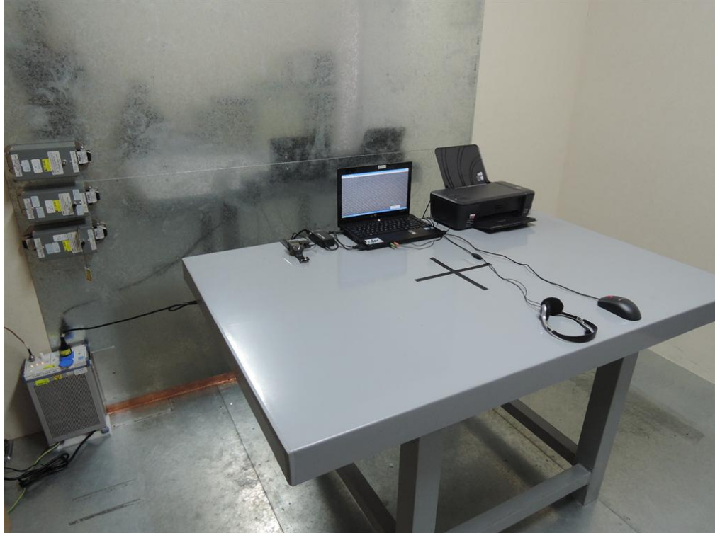
Photograph 6: Set-up for for Mains Conducted testing Front
