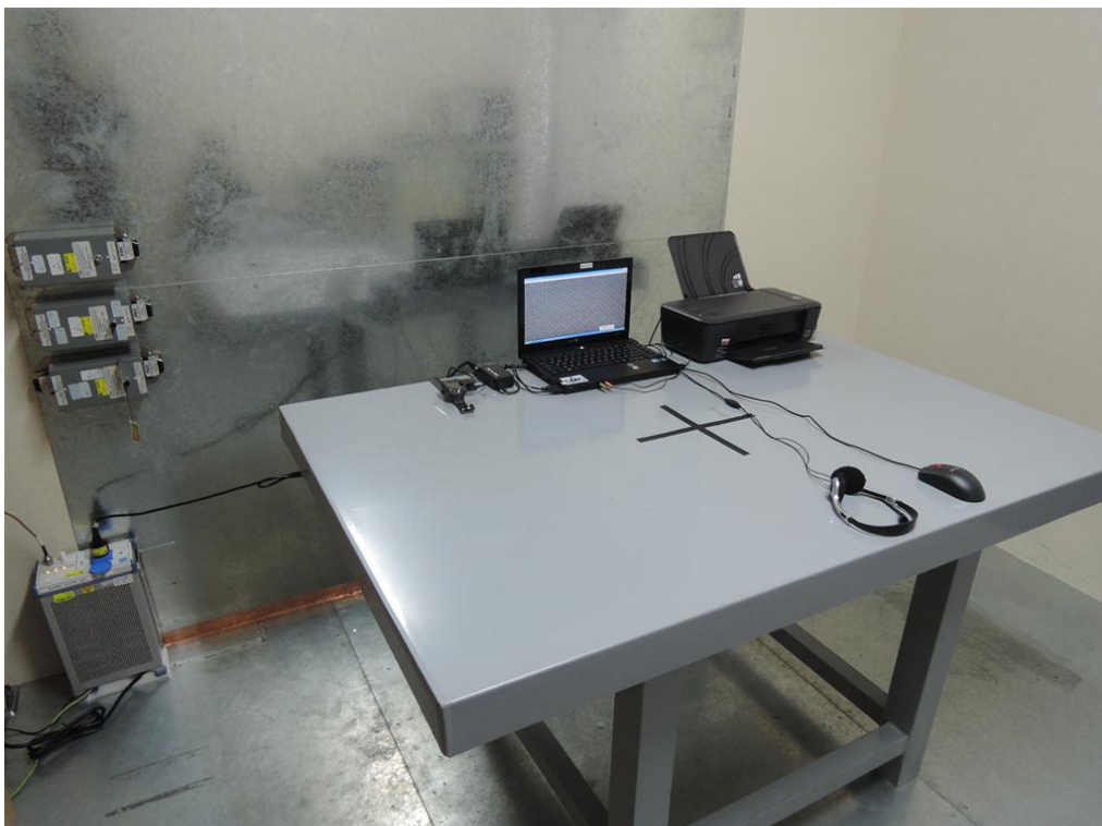
Photograph 6: Set-up for for Mains Conducted testing Front
