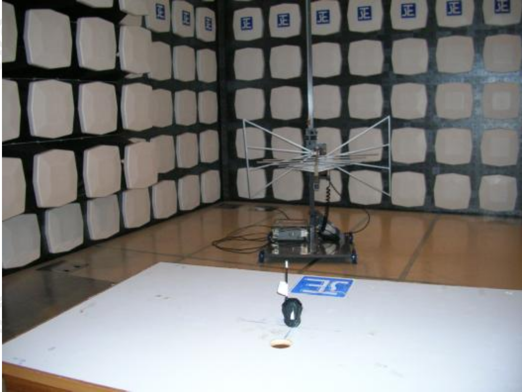
Measurement of Radiated Emission Test Set Up
