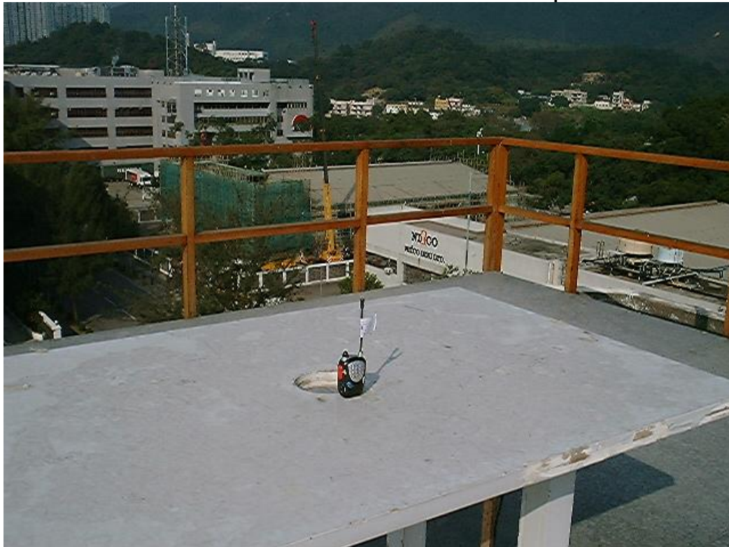
Measurement of Radiated Emission Test Set Up
