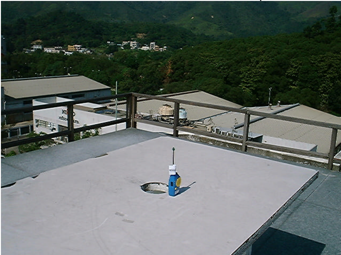
Measurement of Radiated Emission Test Set Up
