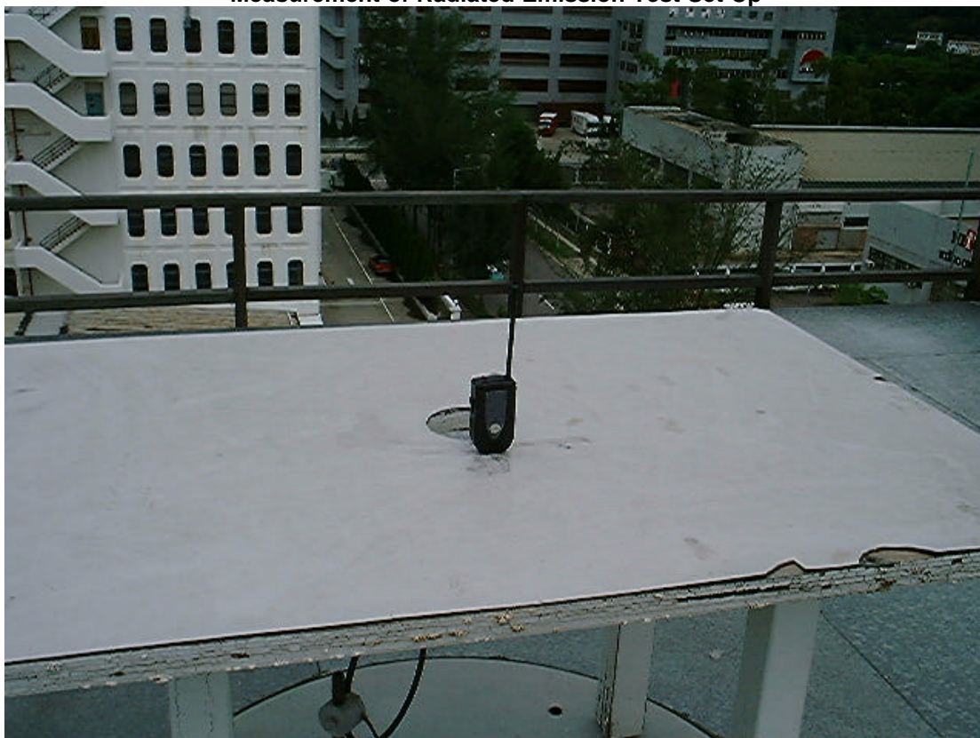
Measurement of Radiated Emission Test Set Up
