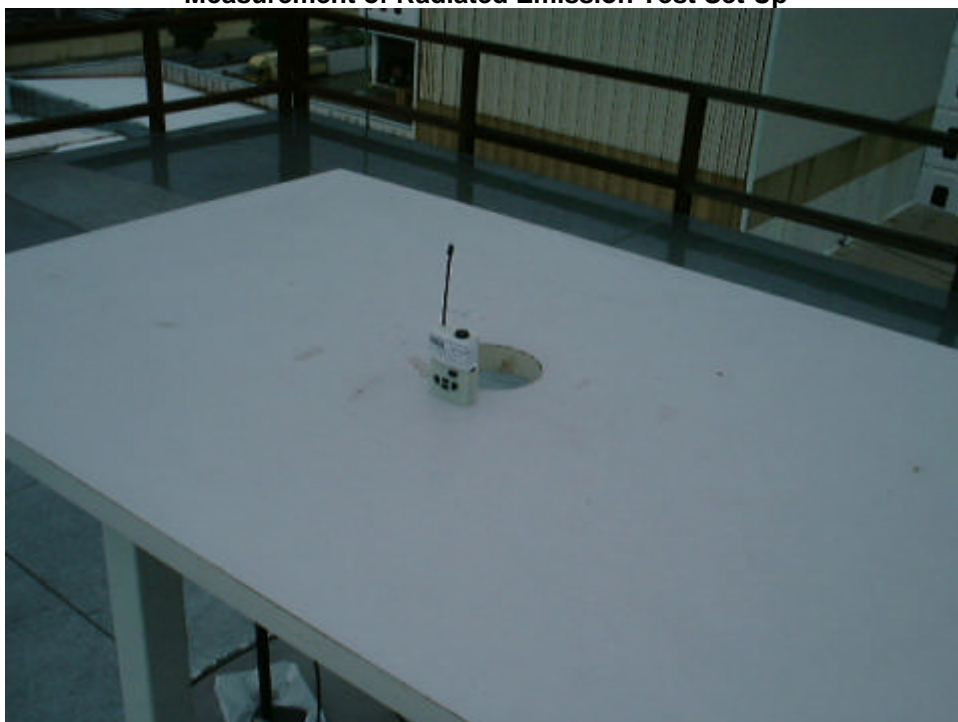
Measurement of Radiated Emission Test Set Up
