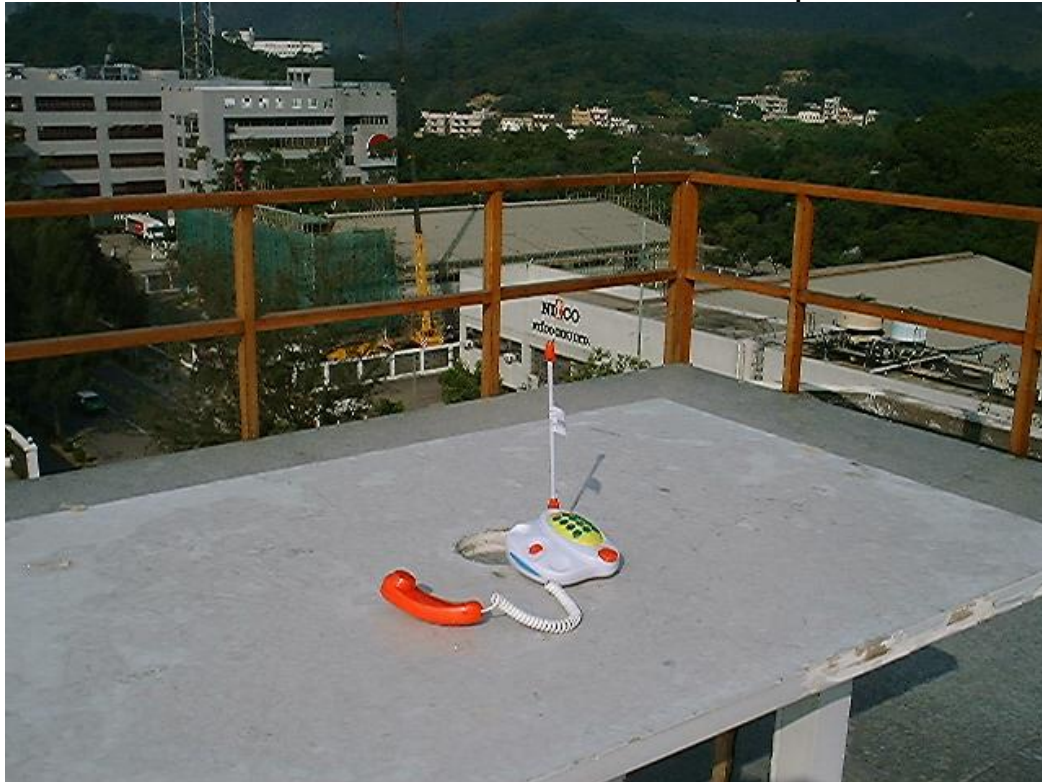
Measurement of Radiated Emission Test Set Up
