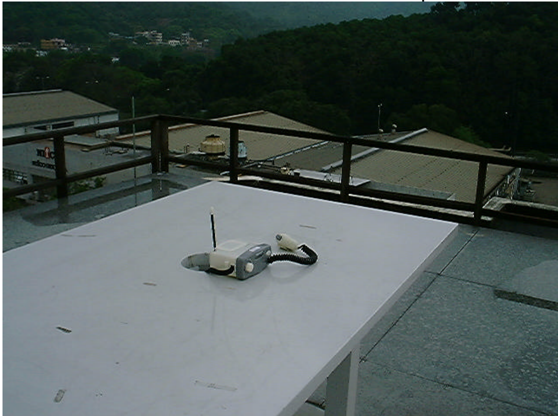
Measurement of Radiated Emission Test Set Up
