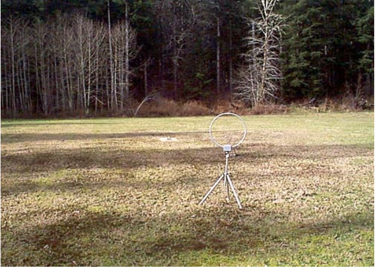
Radiated Emissions - Antenna Below 30 MHz
