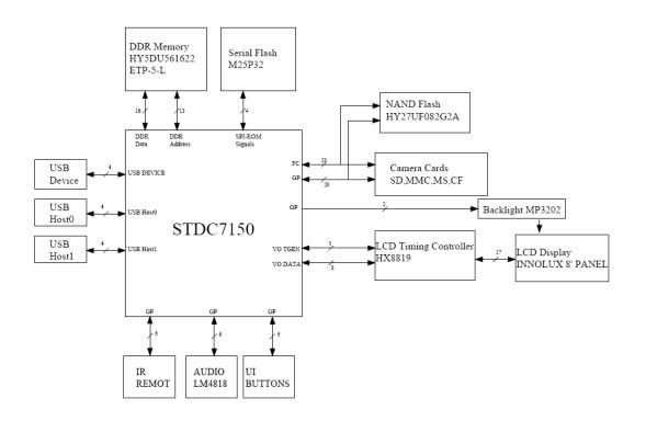
Digital photo frame was made up of several parts including: cpu, ddr, nor flahs, nand flash, t\_con, led panel, card reader, USB interface, remote control and power supply.
