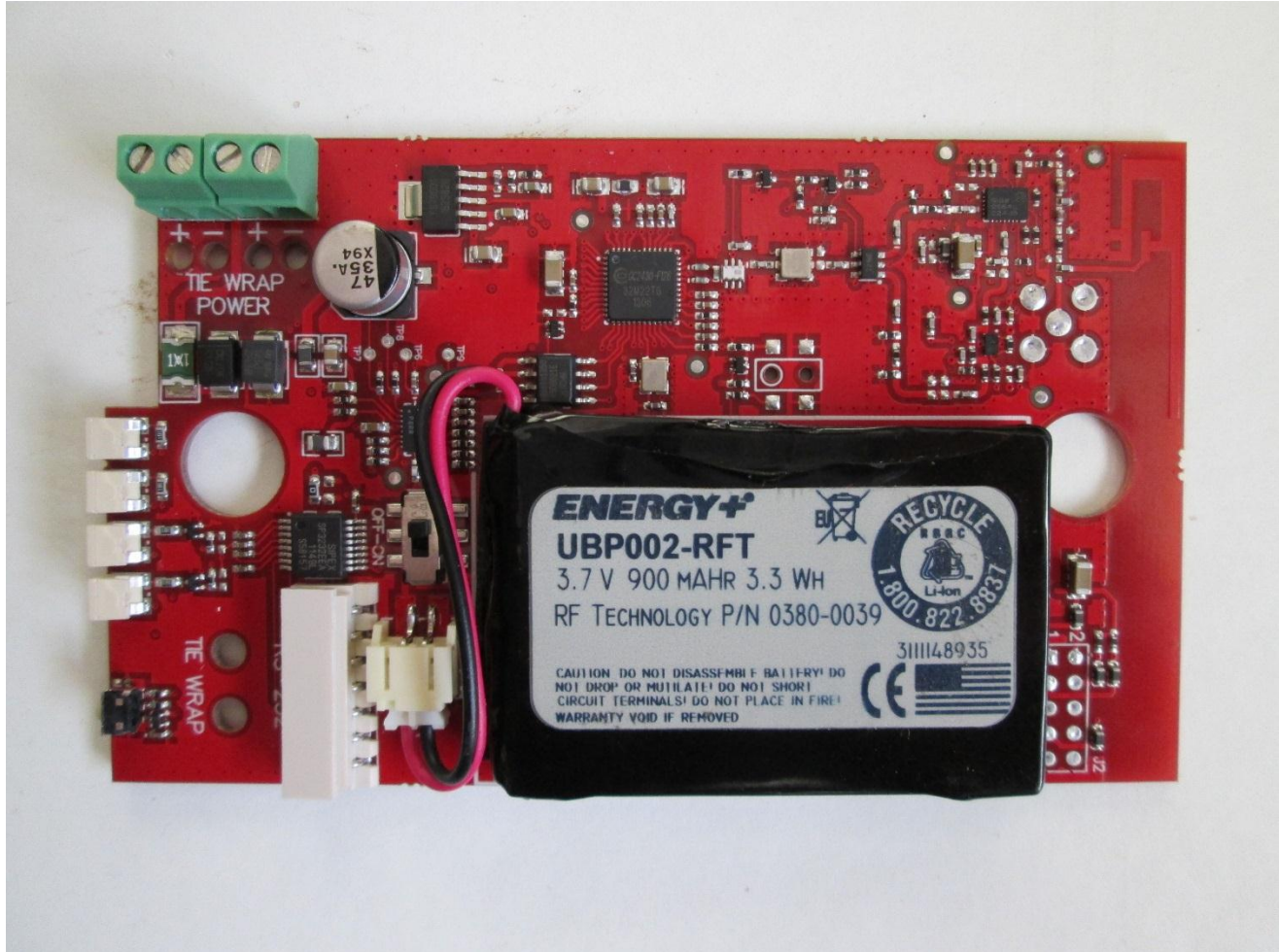
Front Circuit Board Top – with Battery
