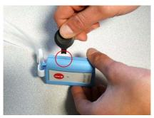
2. If changing the batteries, use a small, non-conductive piece of plastic or wood to pop the battery free from the battery holder.
