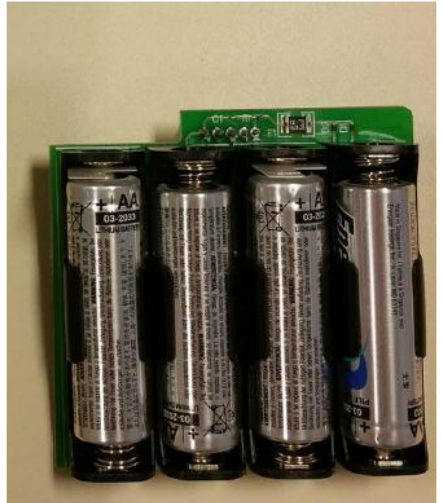
Model 0800-0541 Inside Main Unit & Built In Battery Pack
