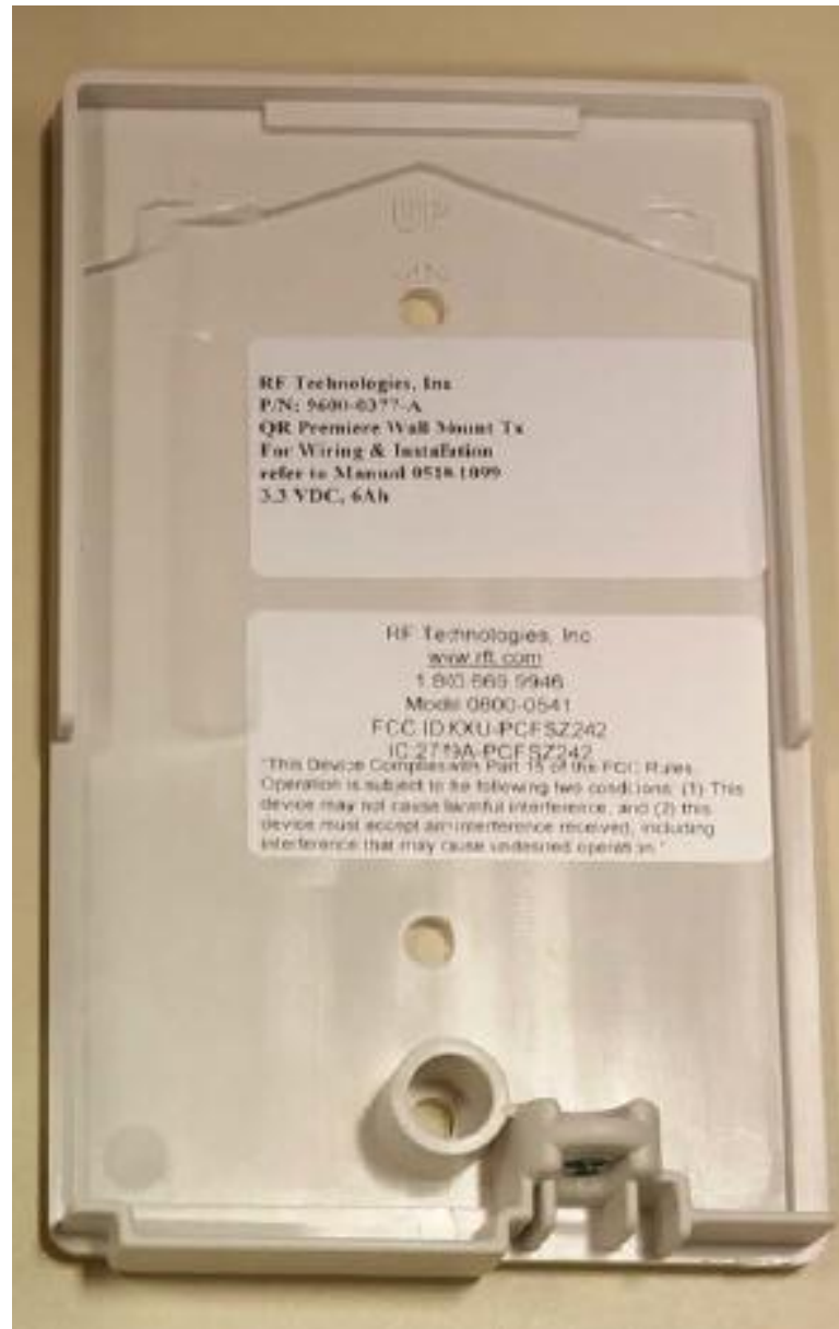
RF Technologies Inc. Quick Response Premiere Nurse Call Push Button & Built In Battery Pack Model: 0800-0541
