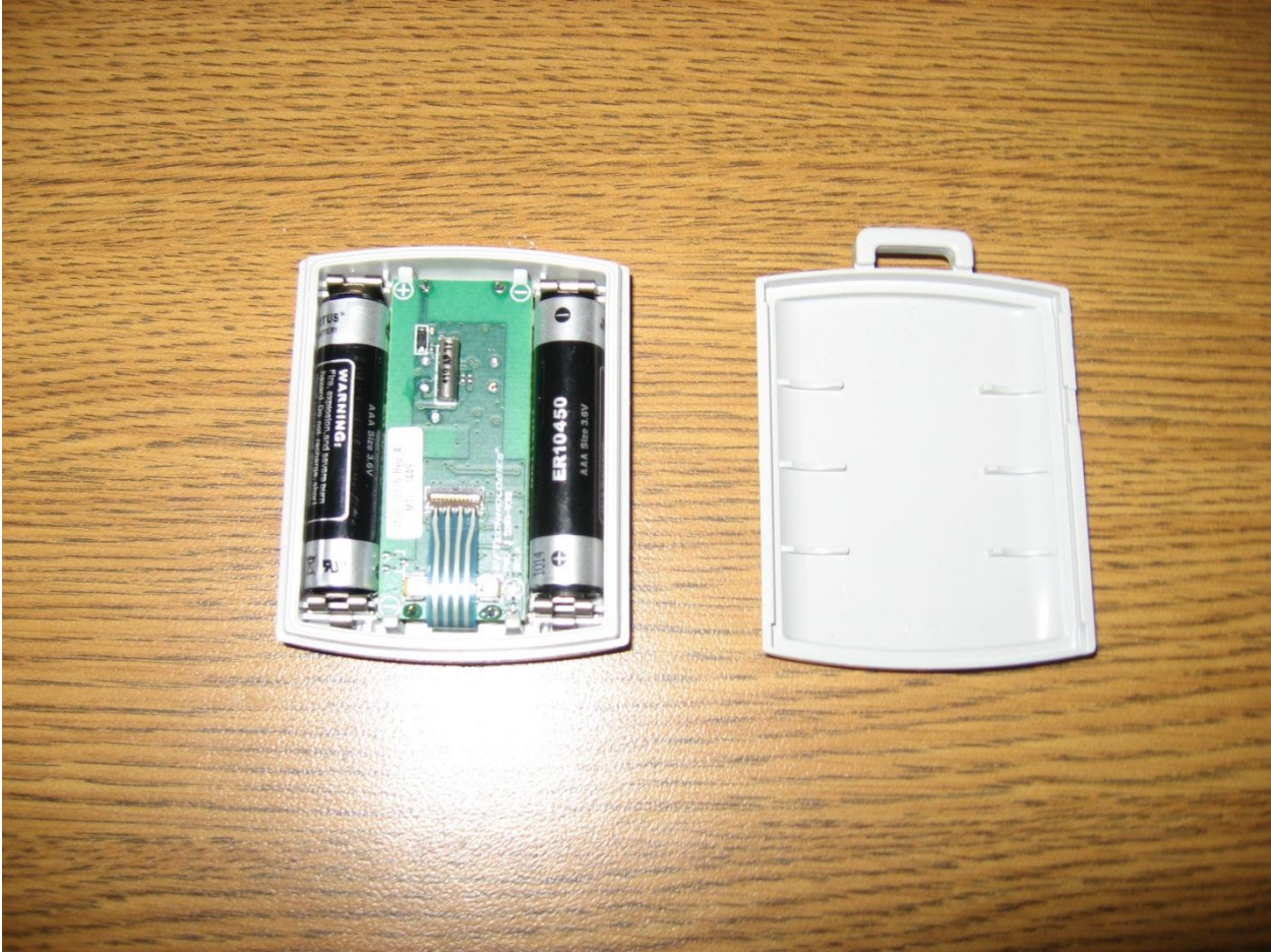
Housing Open with Batteries
