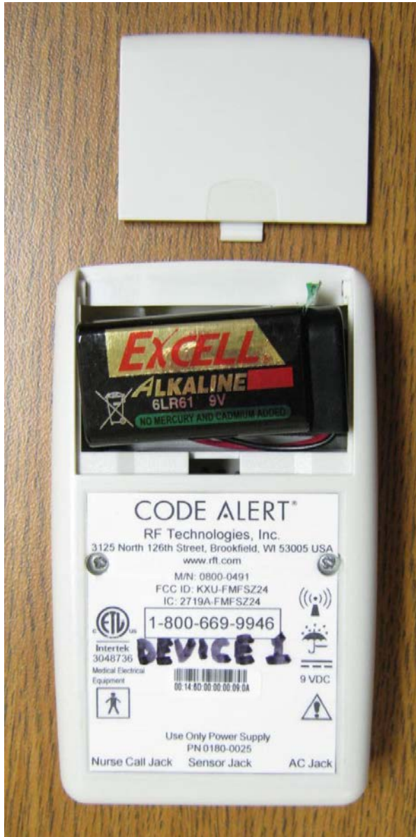
Battery Cover Removed
