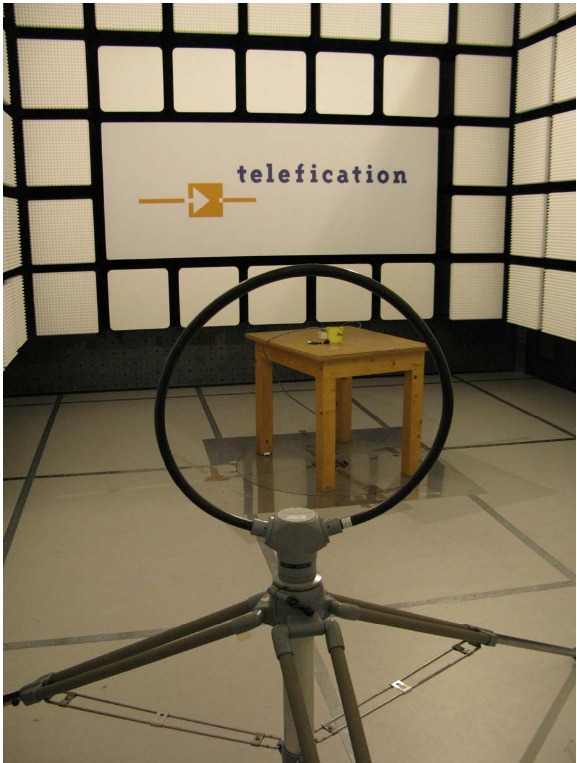
Photograph 1: Test setup radiated emissions (< 30 MHz)
