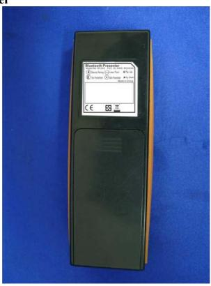
The FCC ID will be placed on the equipment as shown in the photograph below.
