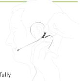
b) Open the loop carefully and attach the iBoom to the left or right ear.
