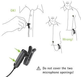
If you are uncertain whether the iLapel is positioned well, activate the Sound check feature in inspiro. Sound check helps to position the iLapel correctly.
