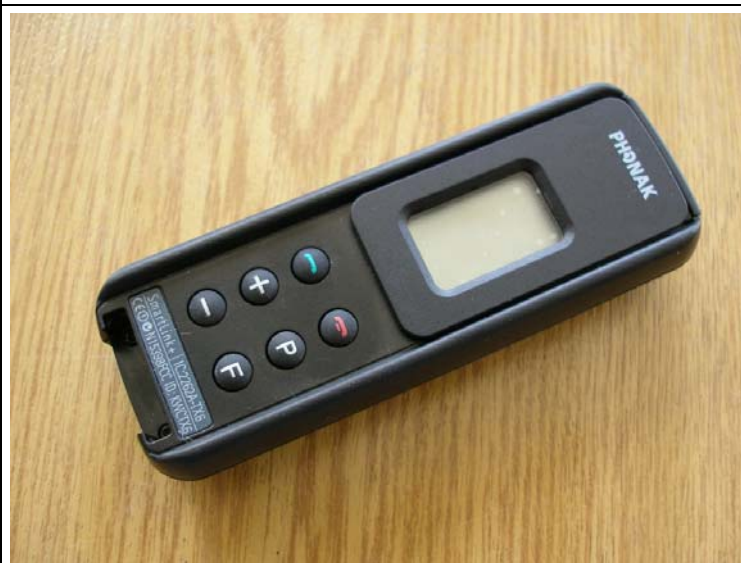
SmartLink+ for radiated measurements (without external antenna)
