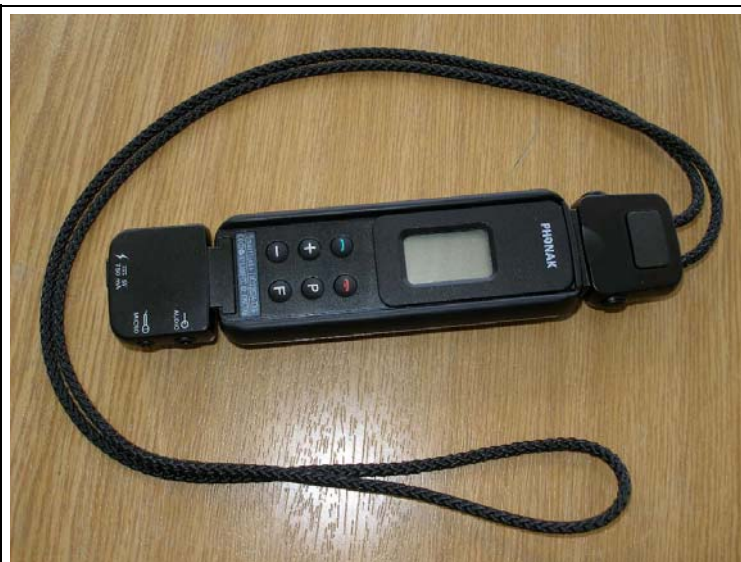
SmartLink+ with adaptor and external antenna
