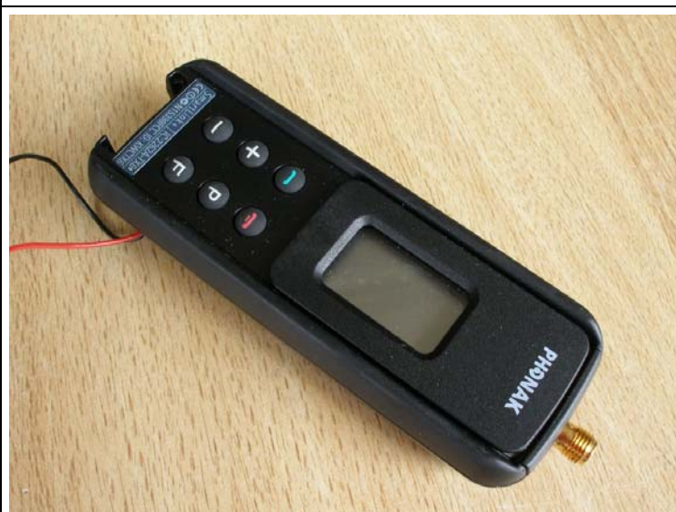
SmartLink+ for conducted measurements (FM part)
