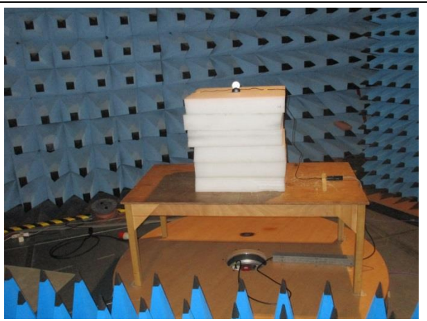
Fig 2 Radiated measurements – carrier and band edge
