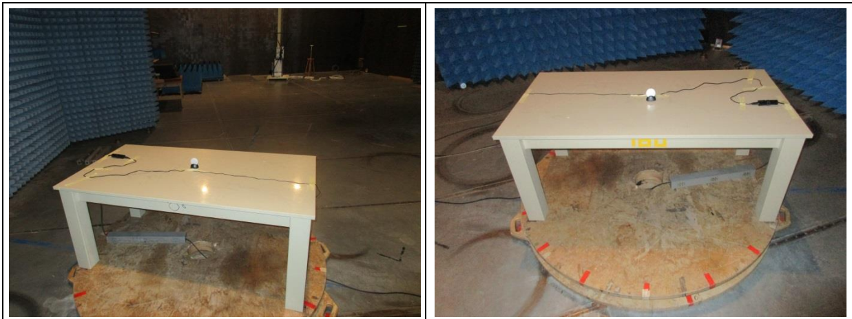
Fig 4 Spurious emissions 30 MHz – 1GHz
