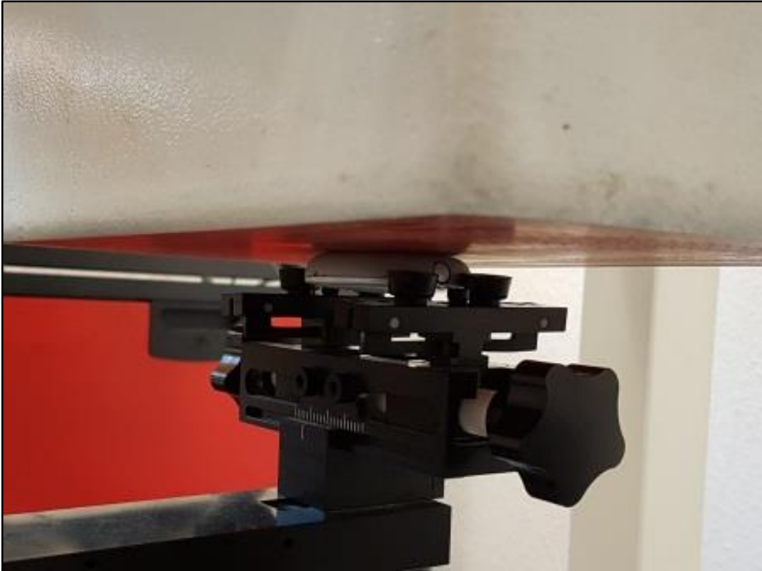
Photo 7: Measurement position - Bottom side with 0mm distance
