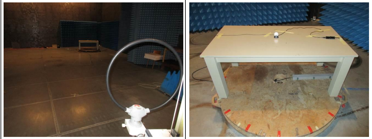
Fig 3 Spurious emissions 9 kHz – 30 MHz
