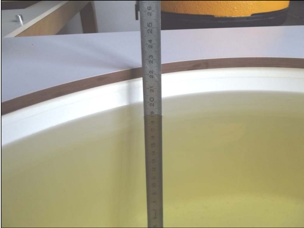
Photo 1: Liquid depth 2450 MHz body simulating liquid
