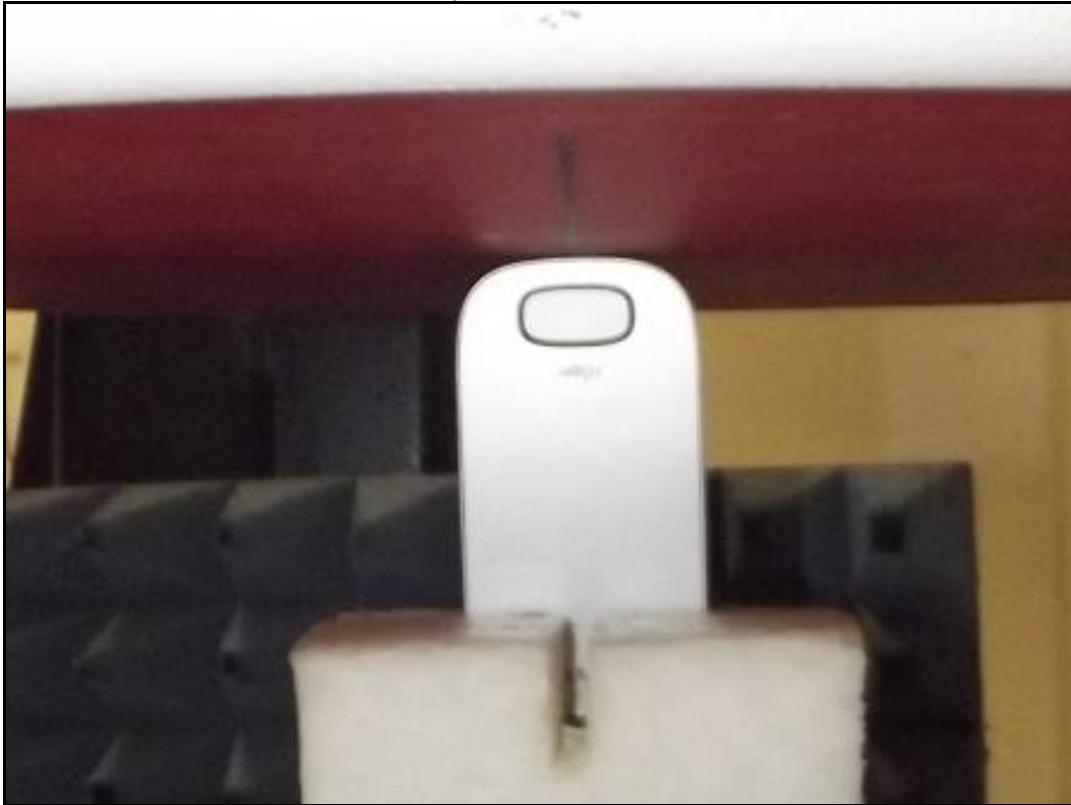
Photo 11: Measurement position bottom side with 0mm distance
