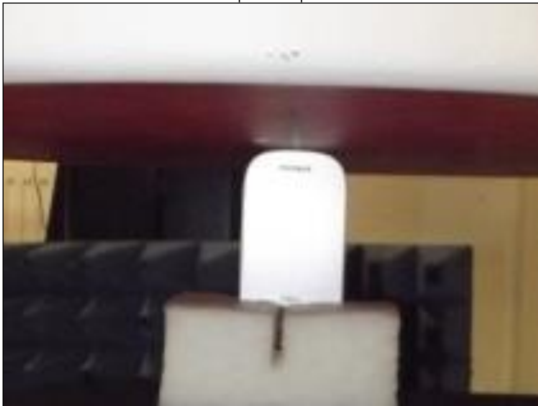
Photo 10: Measurement position top side with 0mm distance
