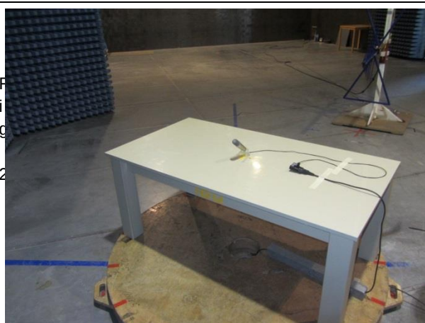
Fig 4 Spurious emissions 30 MHz – 1GHz
