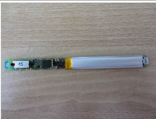
Electronic board (with battery) : front
