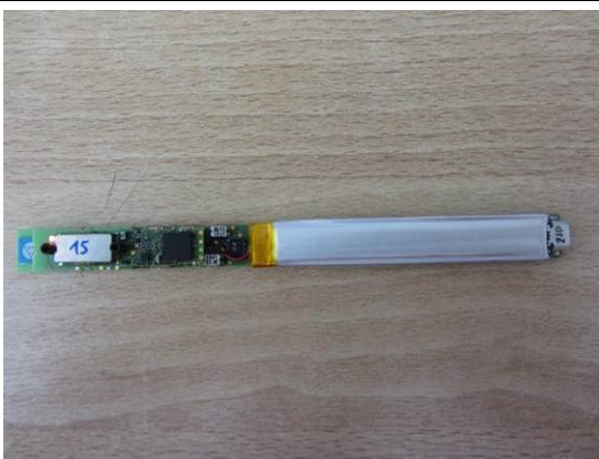
Electronic board (with battery) : front
