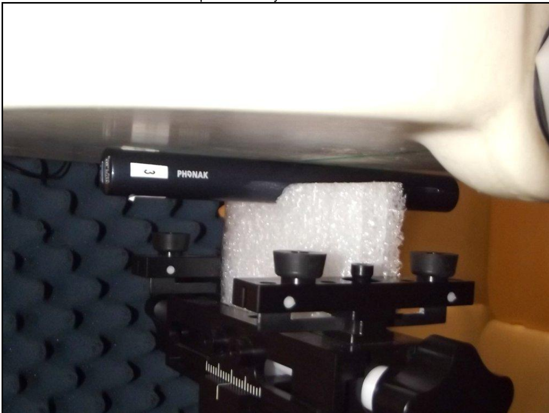
Photo 8: Test position body side3 with 0 mm distance
