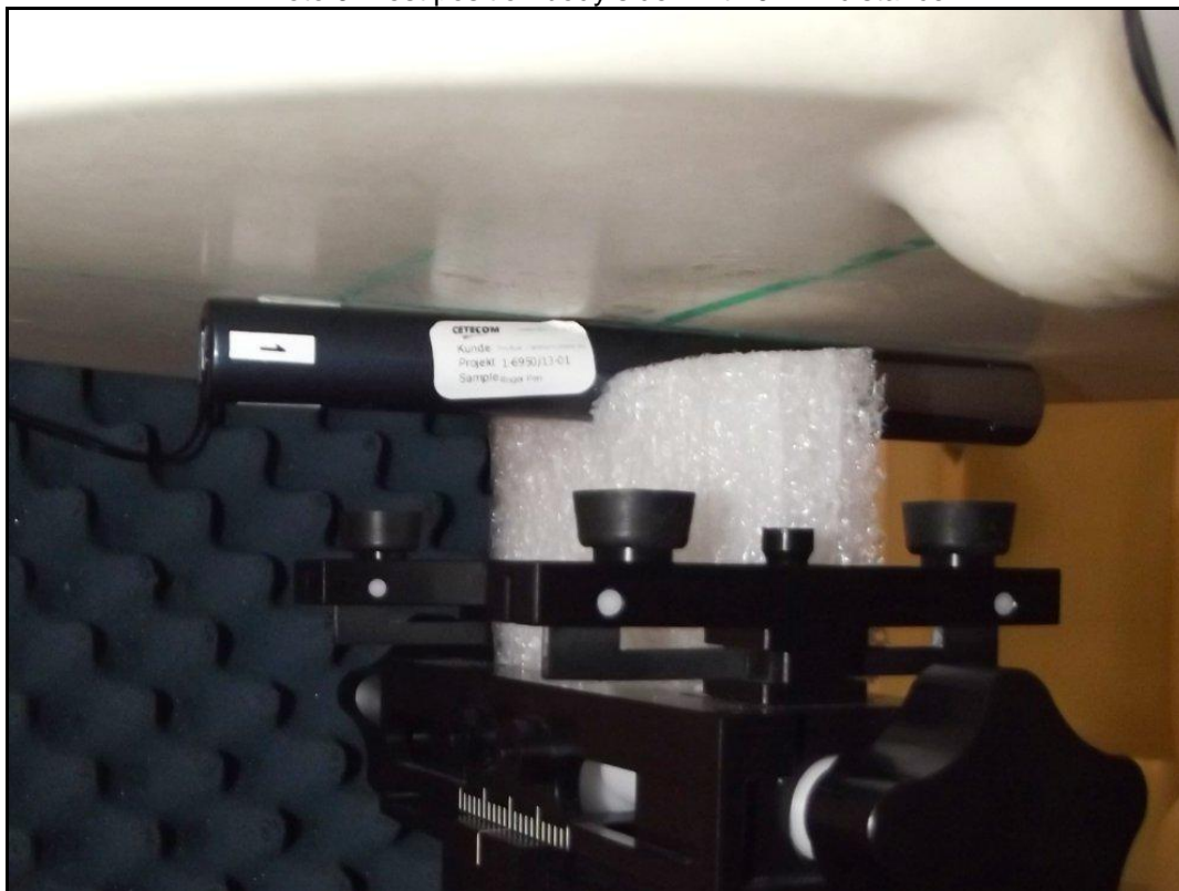
Photo 9: Test position body side4 with 0 mm distance
