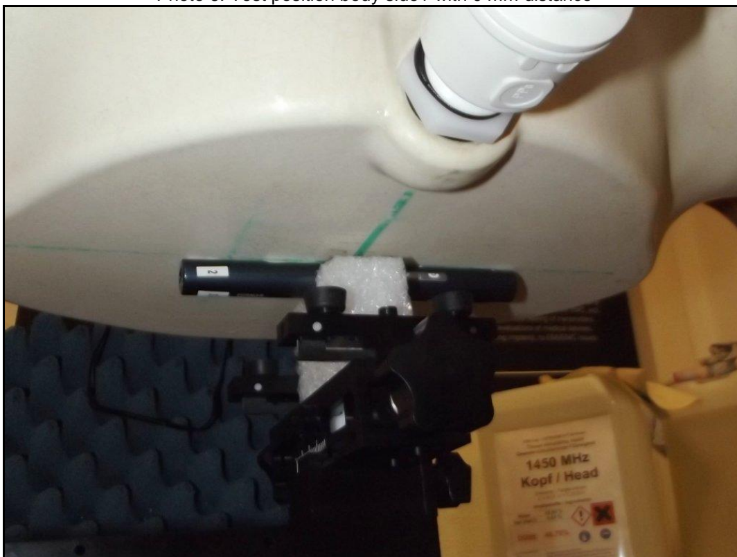
Photo 6: Test position body side1 with 0 mm distance
