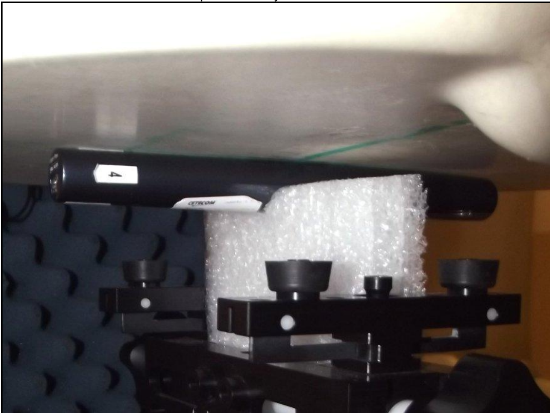
Photo 8: Test position body side3 with 0 mm distance
