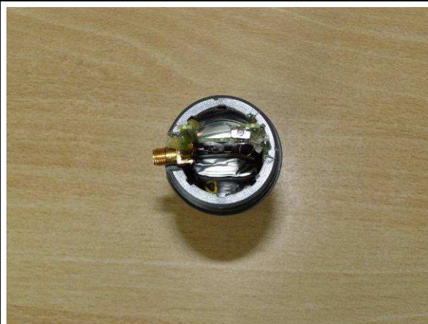
Removed Grid and temporary antenna connector (conducted tests)
