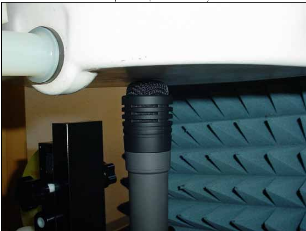
Photo 8: Test position top side without any distance
