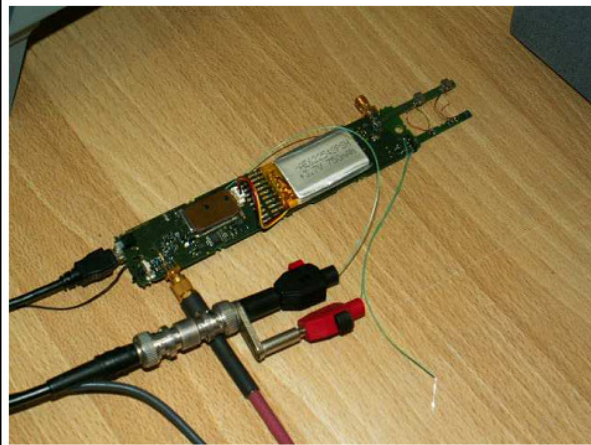
audio injection (green wires)
