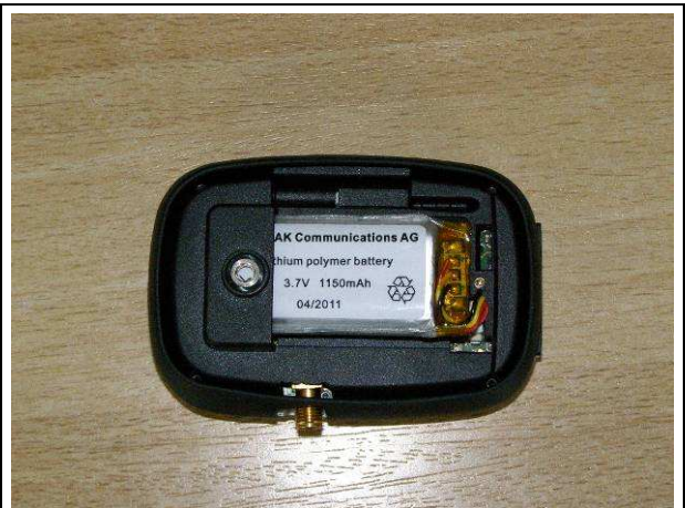
Inspiro 3.0 with temporary external antenna connector back side without battery cover
