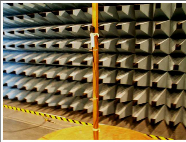
Fig 3 Spurious emissions 1 GHz – 18 GHz
