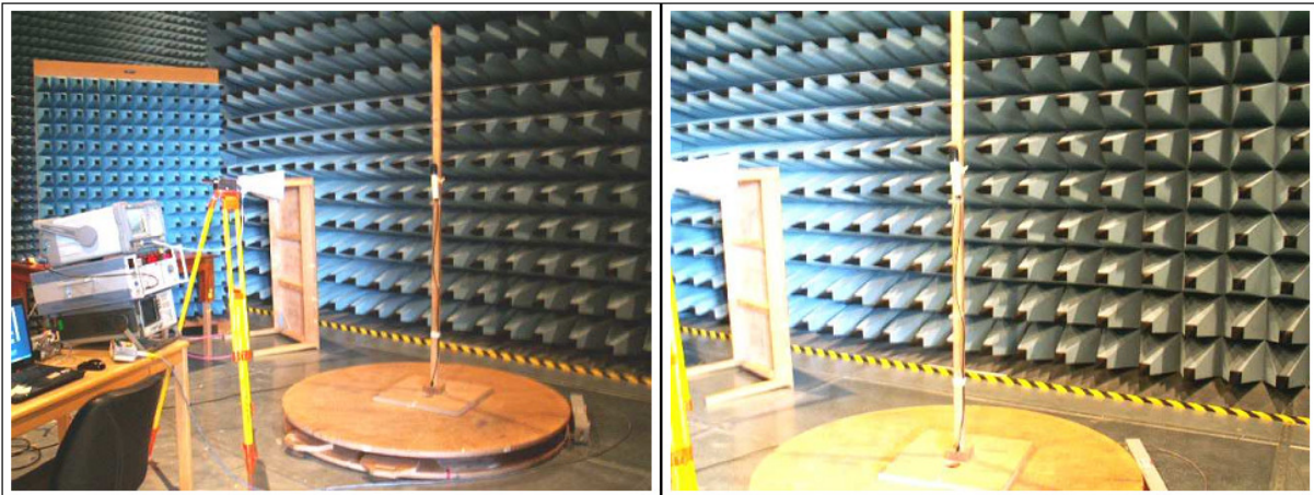
Fig 1 Carrier - radiated measurements
