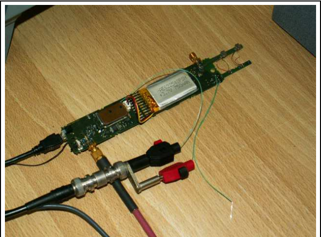
audio injection (green wires)
