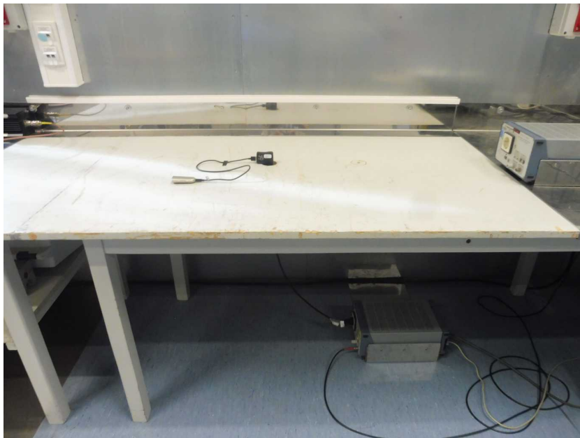
Photo 10: AC conducted test setup
