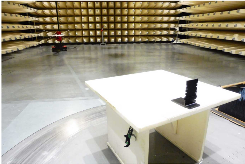
Photo 7: EUT at the semi-anechoic chamber
